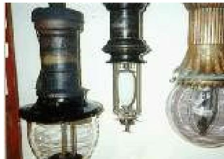
developed in the mid-1890s and limited the operating inside a glass globe which played a major role in increasing the electrodes life to reach almost 125 burning hours.
