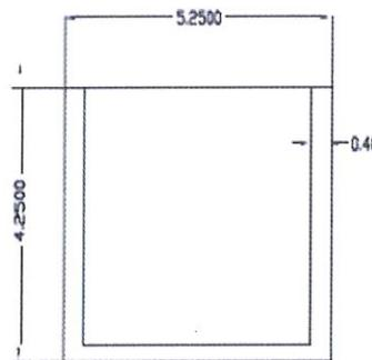
Foundation masonry lay out for family type of shelter
