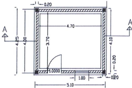
Foundation excavation lay out for family type of shelter
