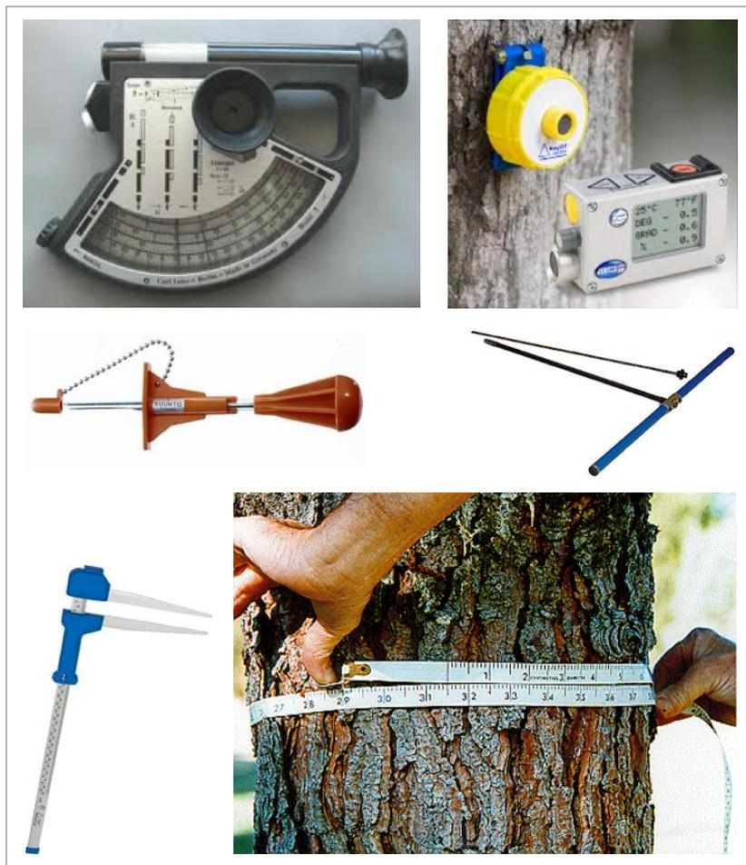
**Figure 15.** Equipment for dendrometric data collection
