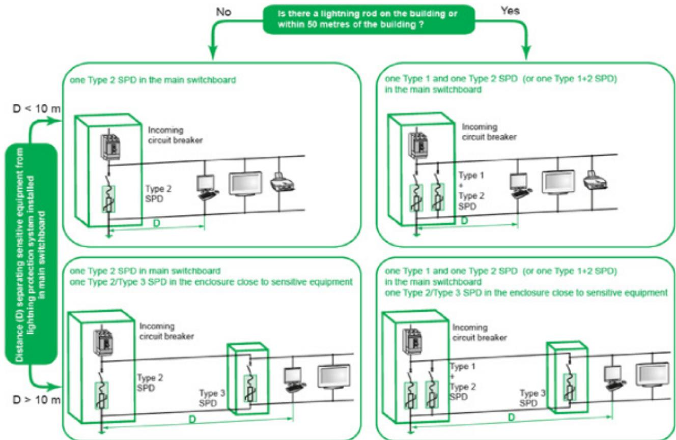
Figure 4: Quick selection guide for SPC (source: Schneider Electric)
