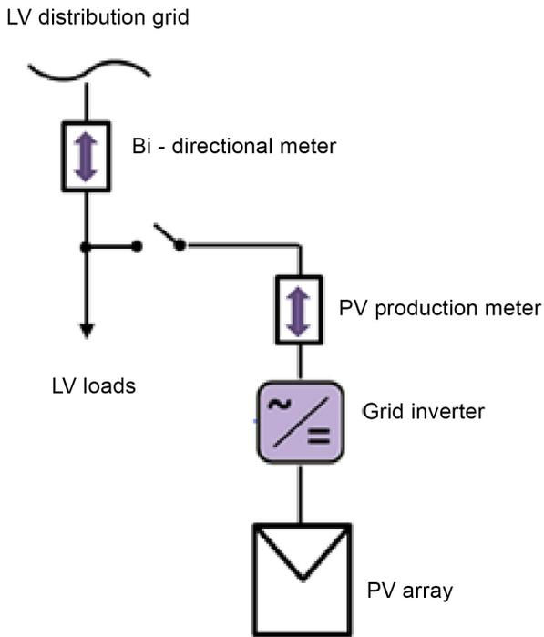
Figure 2: Connection scheme of PV plant for net metering connected to the low voltage grid
