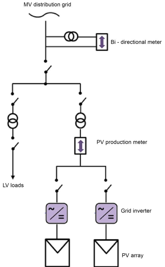
Figure 3: Connection scheme of PV plant for net metering connected to the medium voltage grid
