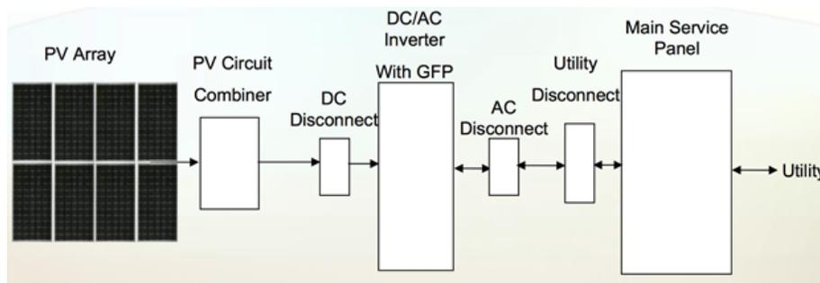
Figure 7: Minimum Equipment Required in the Installation
