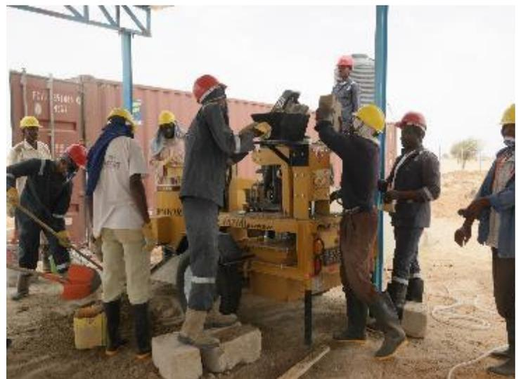
Hydraform machine in action – Brick production with a mix of clay and cement – EU Trust Fund supported project, UNHCR Diffa
