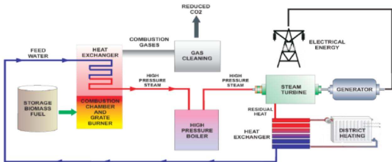
Figure 12. Block diagram of a biomass to CHP (combined heat and power) plant, corresponding to the value chain example presented in figure 11.
