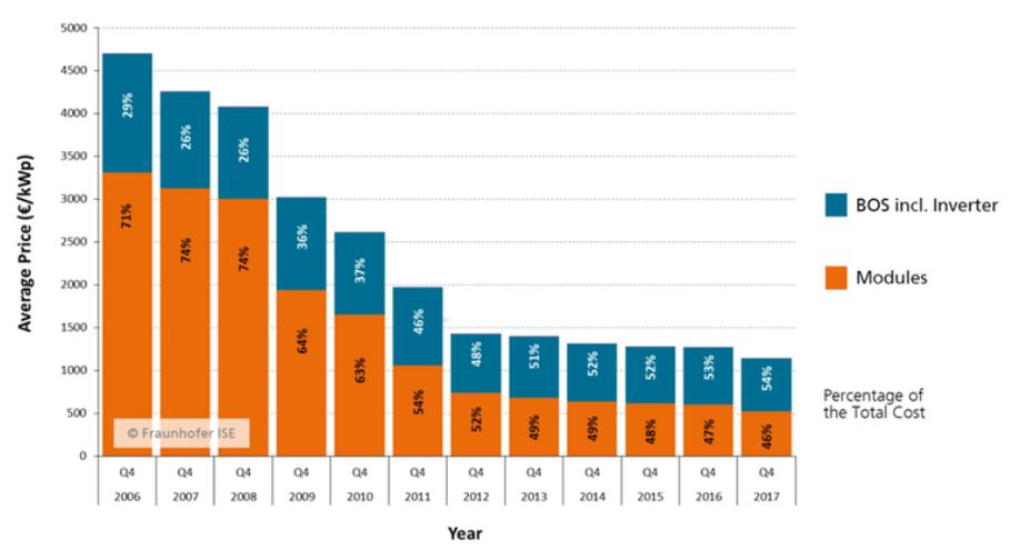
Figure 20. Price development – modules and system costs (Source: Fraunhofer ISE 2017)
