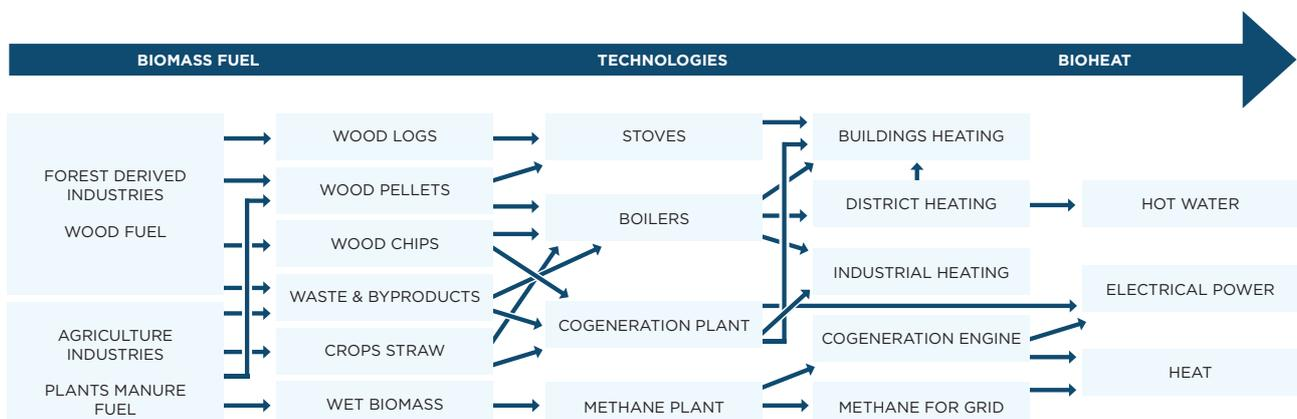
Figure 9. Variety of biomass to heat and power generation pathways
