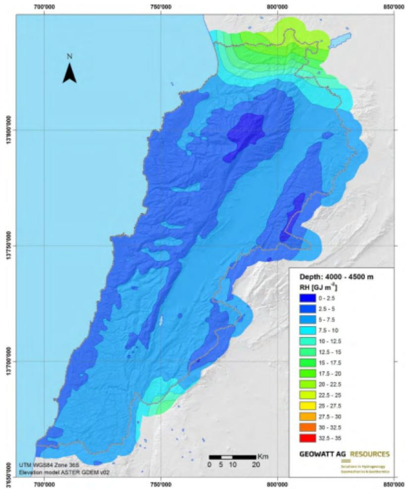
Figure 14. Recoverable heat for the depth interval 4,000-4,500 m
