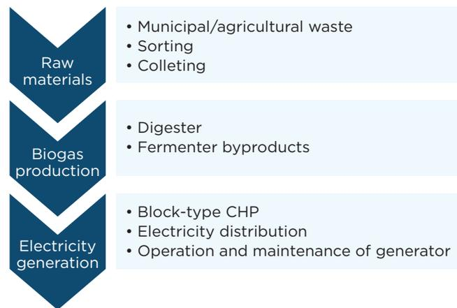
Figure 37. Value chain of Biogas from Municipal waste
