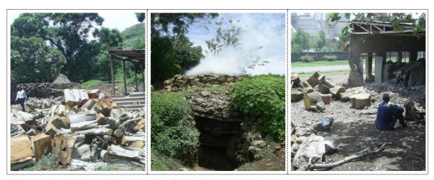
Plate 6.Small scale lime production uses huge logs and tree stumps
