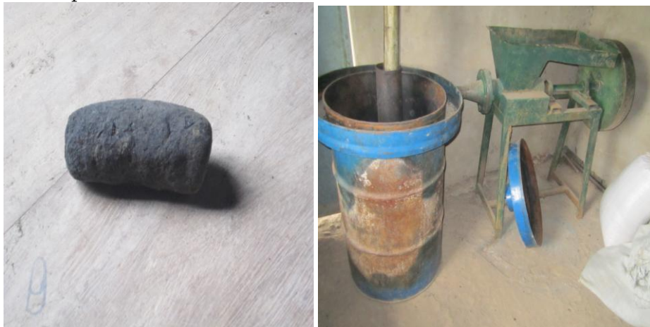
Figure 15: Sample of Charcoal Briquette that has been compressed by a machine in Nakivale.
