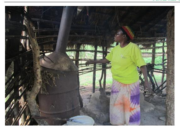
Plate 5: Charring Drum for briquettes
