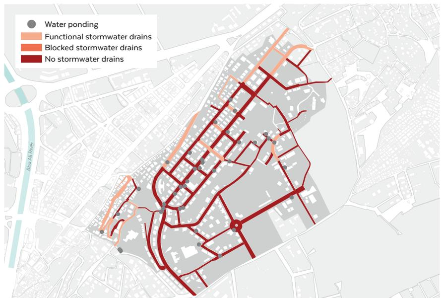
Functional stormwater drains: Drains are functional for stormwater use only, no water ponding.
