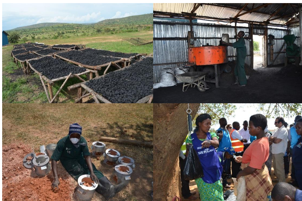
L-R (clockwise): Produced SMBs in the final stage of production-sun drying, ready for use; SMB production plant in Nakivale refugee settlement; a female distributor weighing the briquettes for sale; and a refugee moulding clay for lining the metallic iron sheets fabricated into energy saving stoves. © UNHCR/E.Ohanusi, August 2015.
