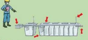
Check vessel quality: condition of manhole cover, gas release, inlet and outlet pipes, and condition of the wastewater treatment installation divider walls (look for cracks and leaks).
