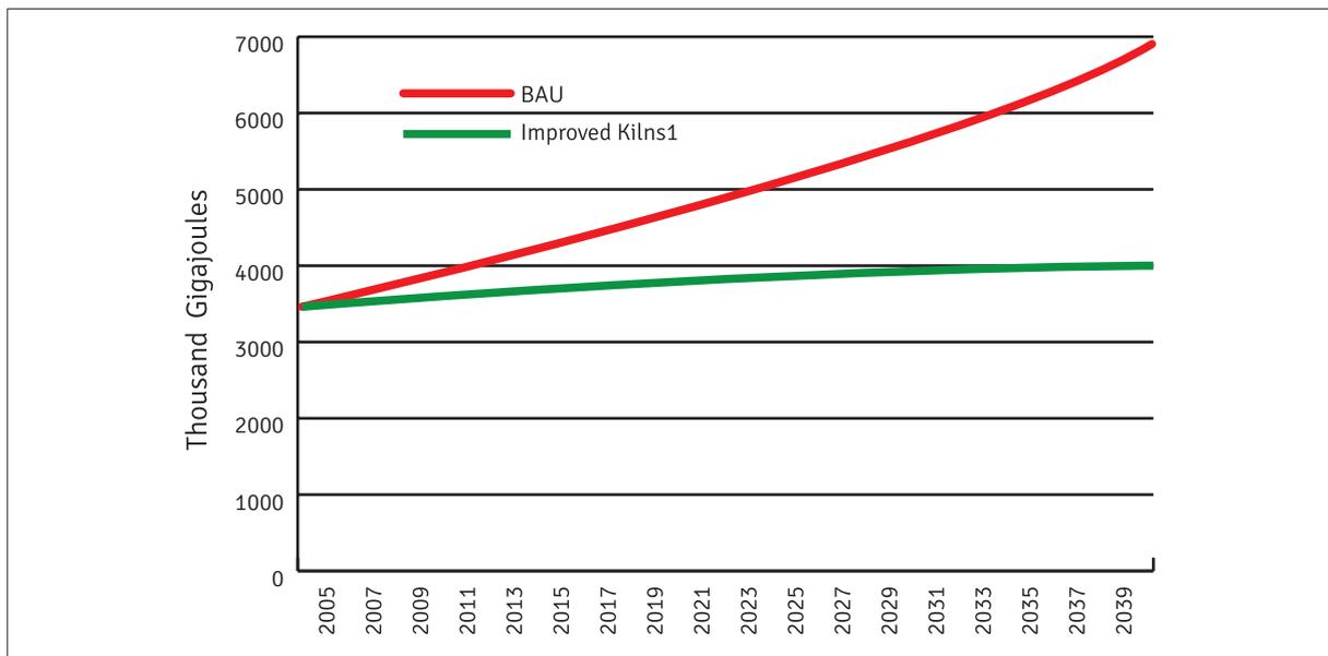
Figure 14 Lime Potential energy (wood ) savings in the lime industry (1 tone wood = 15GJ)
