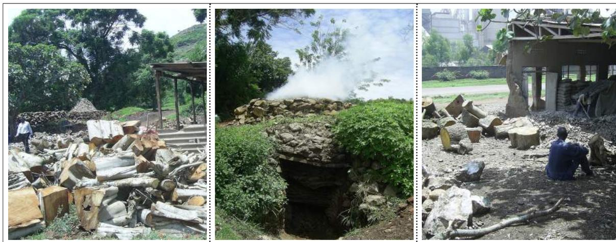
Plate 6. Small scale lime production uses huge logs and tree stumps
