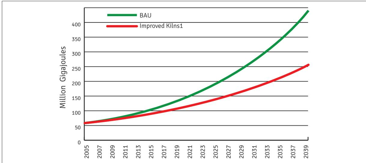
Figure 15. Potential Energy (wood) savings in the brick baking industry (1 tone of wood = 15 GJ)
