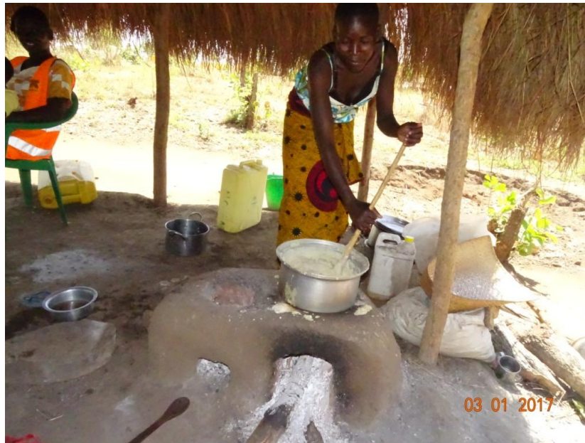
Figure 11. A woman cooks posho (maize meal) on an improved mud stove (two-pot rocket lorena)
