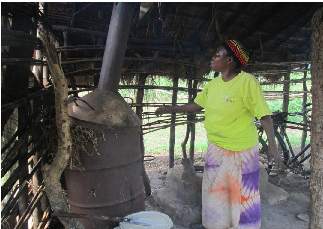
Plate 5: Charring Drum for briquettes
