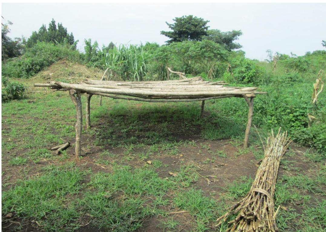
Plate 4: Drying rack used to dry Briquettes produced by Wandaleyo Group
