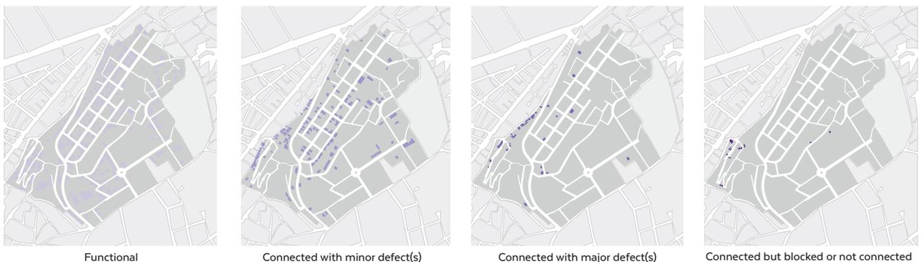
Figure 46 Condition of buildings' connection to wastewater network
