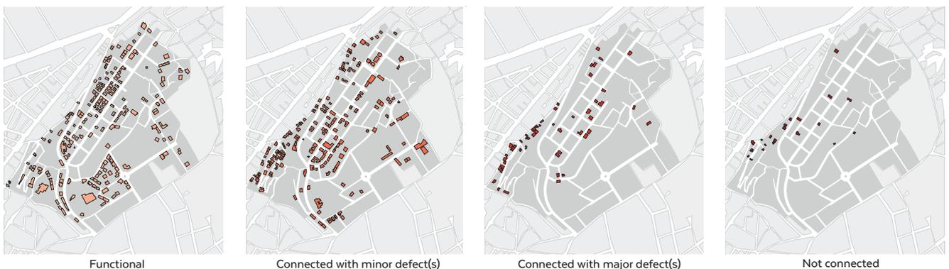
Figure 48 Condition of buildings’ connection to stormwater network
