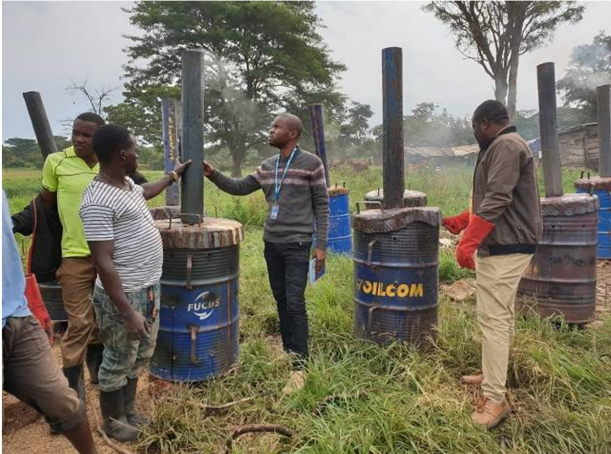
Figure 11: Metallic kilns used for charcoal production at one of charcoal production sites in Mvugwe village in Kasulu District © UNHCR
