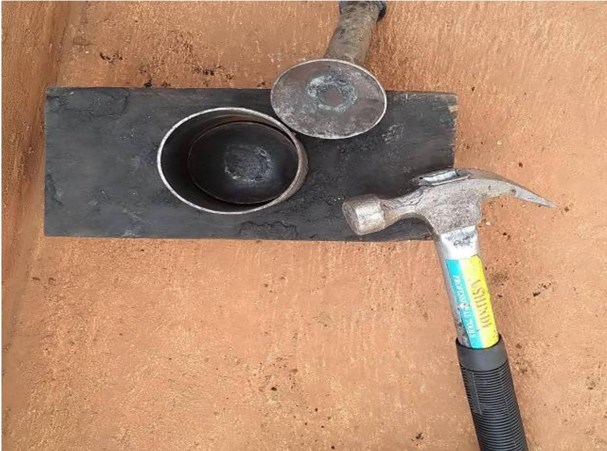
*Figure 12: Manual pressing tools used to produce the charcoal briquettes in the community-based charcoal briquettes production in Nyarugusu Camp.*
