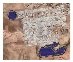
The available land within the camp is flat and unshaded and requires limited earthworks making it highly suitable for the installation of a PV-power plant. The site has easy access and there is sufficient labor available for construction and maintenance of the plant.
