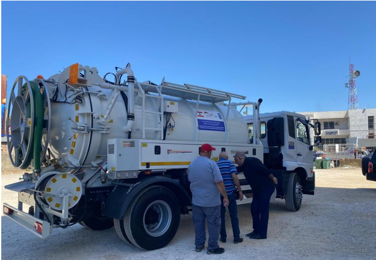
Figure 4. Sewage & Jetting truck provision to Chtoura Municipality for sewage desludging and opening & cleaning clogged water canals to prevent flooding in winter, by UNDP. © UNDP.
