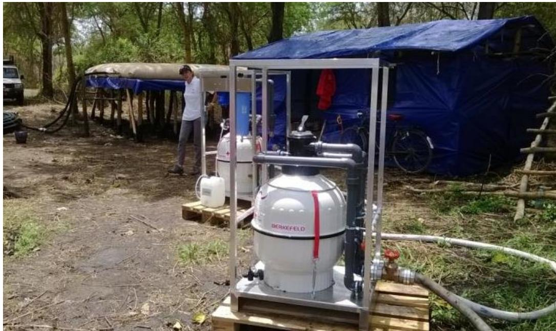
**A water purifying system near River Enyau is providing clean water for trucking to Rhino Camp settlement. The kit was supplied by the German Red Cross and is being operated by the Uganda Red Cross Society. ©UNHCR/ A. Ndungu**
