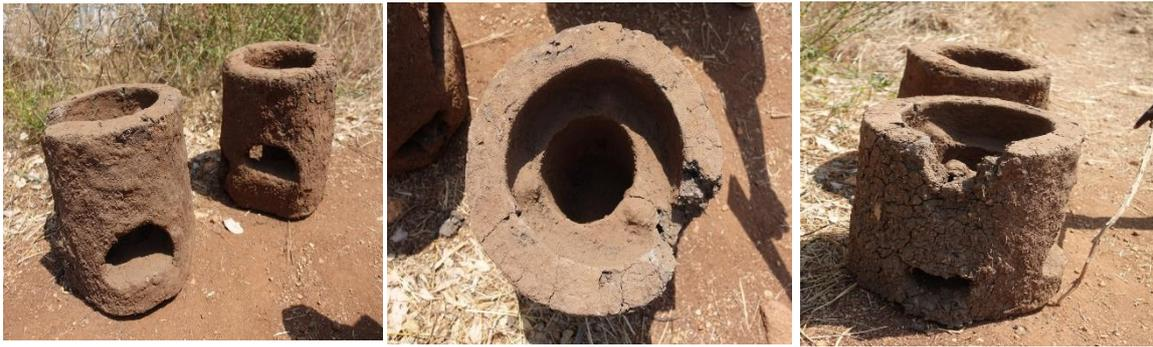
*Samples of Local Mud Stoves made by ToTs Trained by GiZ showing cracking and broken saucepan cavity*
