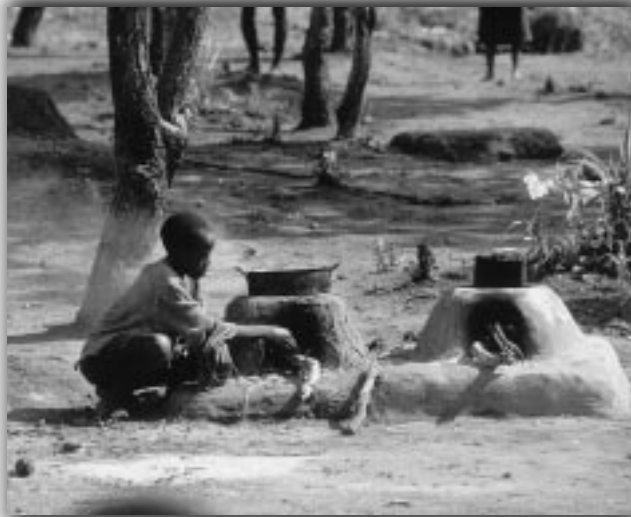
Fuel-efficient stoves, made from clay or metal, use less wood than traditional three stone fires and thereby help reduce pressure on the environment surrounding camps. UNHCR/C. Sattlberger
