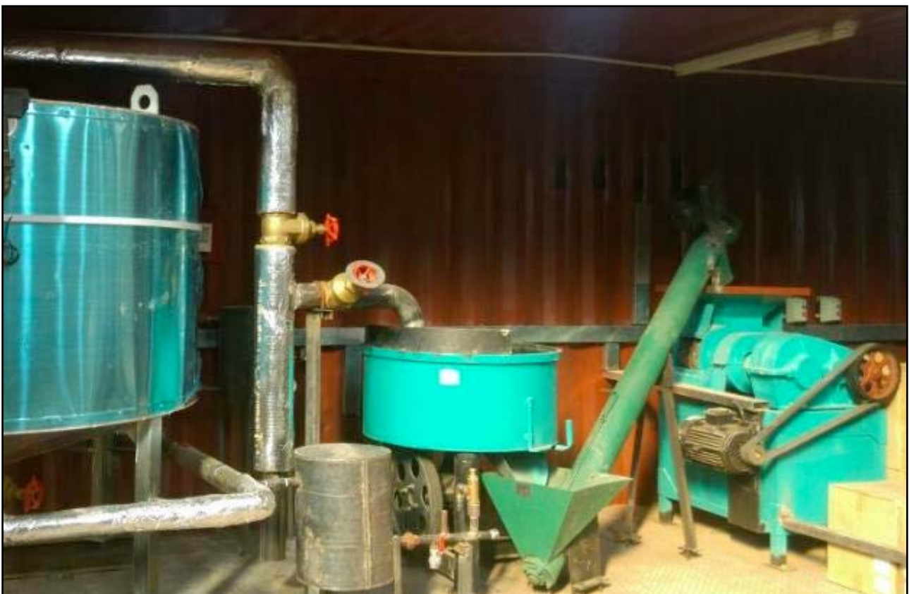
Figure 12 - Treatment and reuse system comprising treatment tank, mixer, conveyor and roller press
