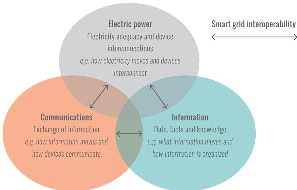
Figure 4: Relations amongst electric power, communications and information in the smart grid (Basso, 2014)
