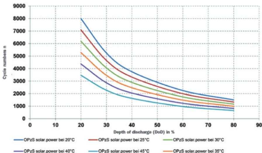
Figure 6: Lifetime of OPzS batteries (in cycles) for different temperatures and DOD levels (source: Hoppecke)
