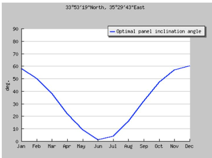
Figure 11: Optimal panel inclination angle per month for Beirut (source: PVGIS)
