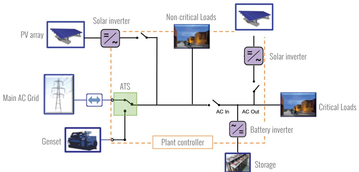
Figure 1: Architecture of a grid and genset inter-connectable PV plant
