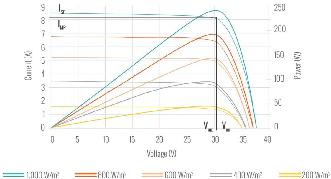
Figure 7: Combined I-V and power output curve of a 245 WP polycrystalline module at AM 1.5 and 25°C (source: Suntech)
