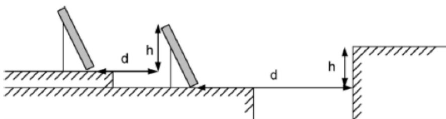
Figure 12: Variables to calculate the minimum distance between PV arrays (IDAE and CIEMAT, 2002)
