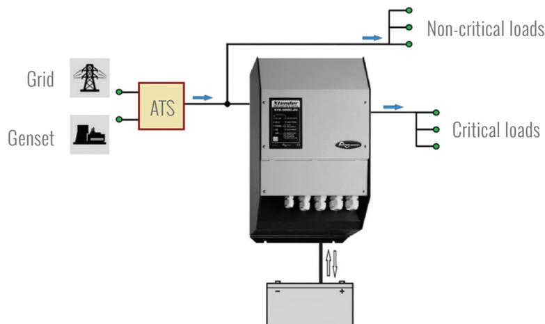
Figure 10: Dual mode inverter with external ATS (source: Studer Innotec)
