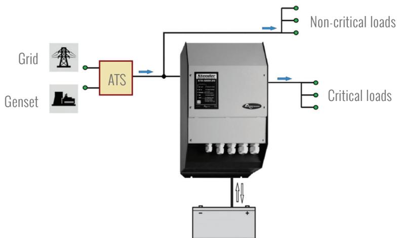
Figure A4: Dual mode inverter with external ATS (source: Studer Innotech)
