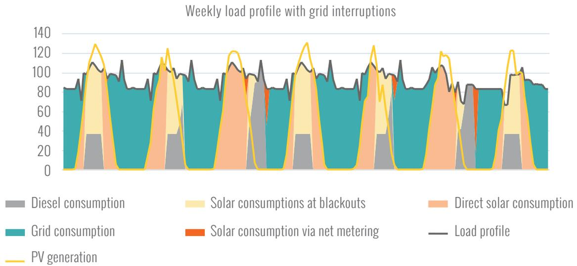
Figure A2: Sample of a weekly load profile with grid interruptions
