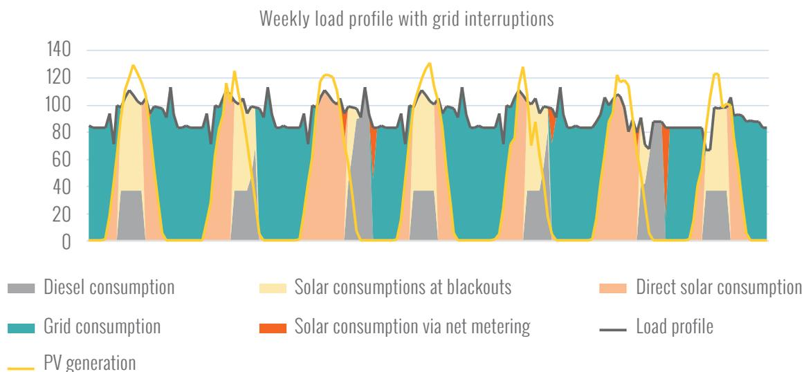
FigureA1-1. PV-hybrid plant operation during a random week with persistent grid interruptions (source: TTA)
