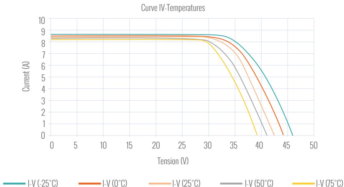
Figure 8: I-V curve for different temperatures of a 300 Wp polycrystalline module (source: Solar Innova)
