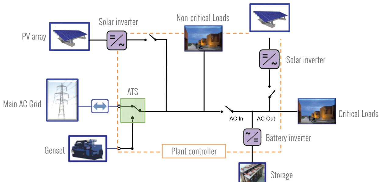
Figure A1: Overview of the PV-hybrid plant with PV and genset generation, storage and a PV plant controller
