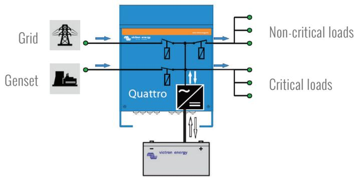
Figure 9: Dual mode inverter with internal ATS (source: Victron Energy)
