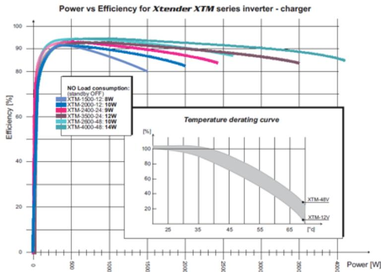
Figure 13: Efficiency derating curve of a dual mode inverter (source: Studer Innotec)
