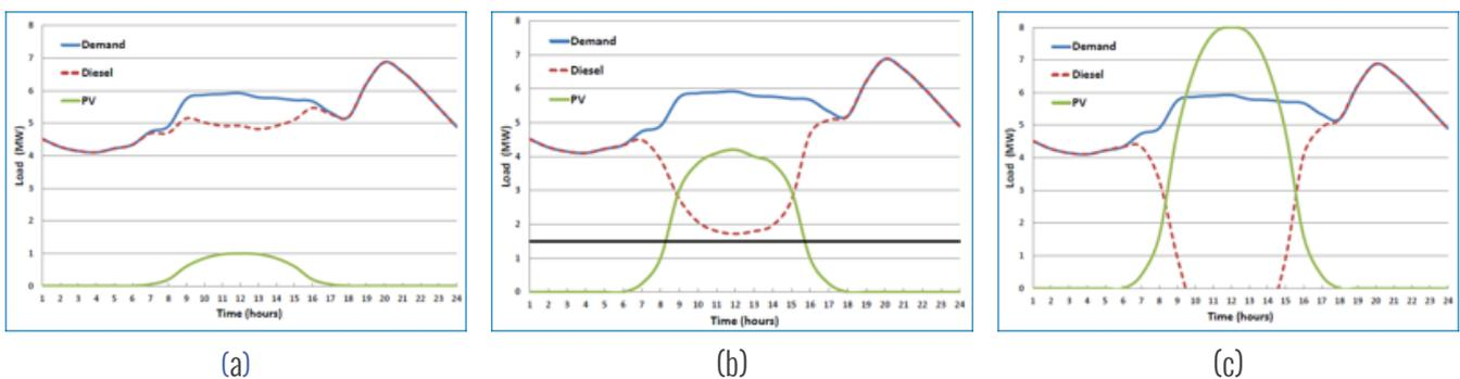
Figure 3: Simulation of a low (a), medium (b) and high class (c) fraction levels of PV (source: UPC)
