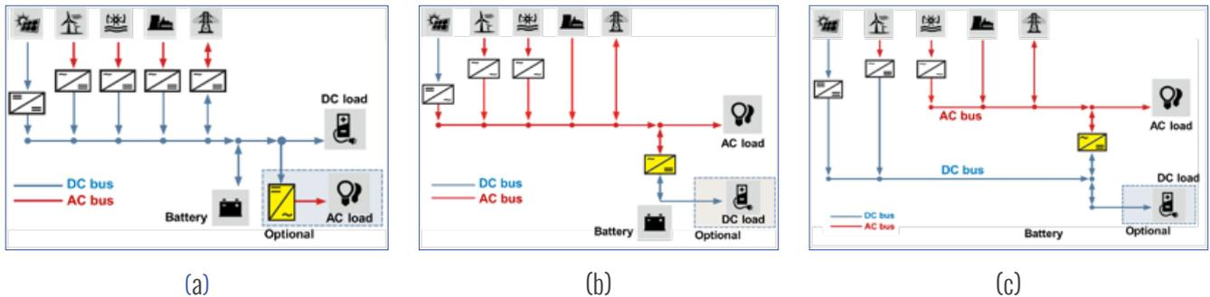
Figure 5 : Configurations with a DC (a), AC (b) or mixed AC/DC (c) coupling (source: UPC)
