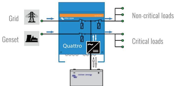
Figure A3: Dual mode inverter with internal ATS (source: Victron Energy)
