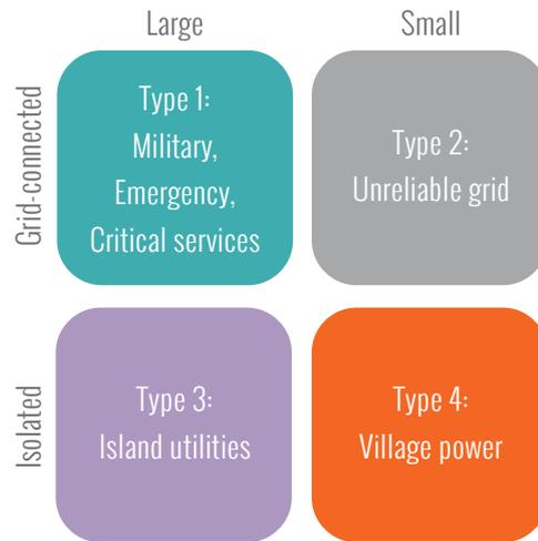
Figure 2: Microgrid classification (source: HOMER Energy)
