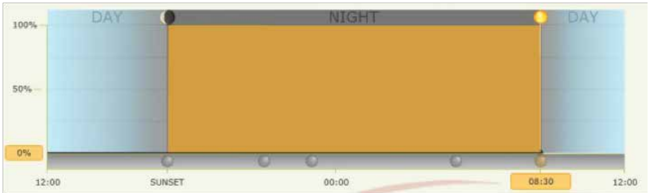
Figure8: Typical on-off timer operation profile
